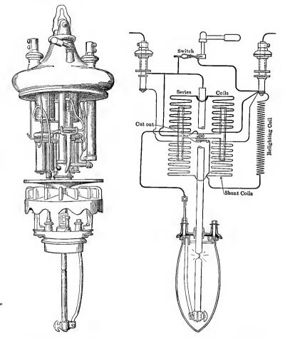
FIG. 4. View and diagram of the carbon arc lamp in which light is produced by the heat generated in the arc.
